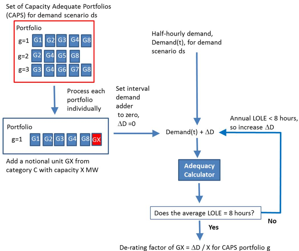
Figure 6: Schematic of the Marginal De-Rating Approach
