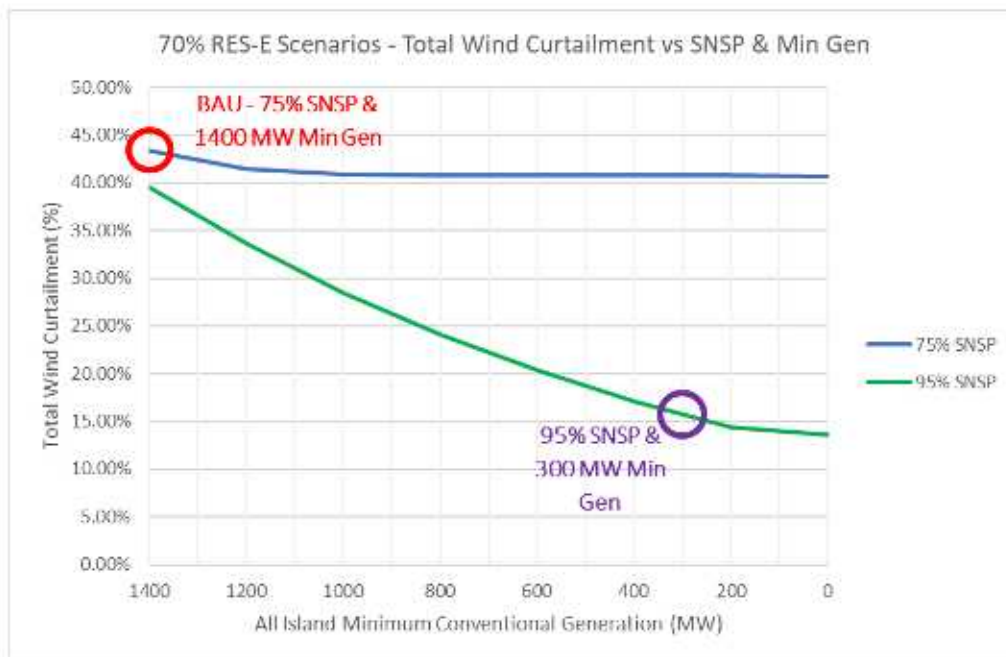
Figure 1: Curtailment vs minimum system conventional generation for 75% and 90% SNSP limits for 70% RES-E systems (Both lines represent a 70% RES-E system with the level of curtailment related to changes in Min Gen levels, all other system assumptions based on 2020 system).
