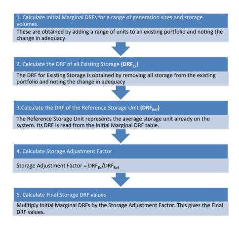
De-rating curves are produced based on size and storage durations. There will be a set of de-rating curves for pumped hydro storage units (based on its historical outage statistics) and another set of de-rating curves for other new storage types (such as batteries, compressed air and flywheels) that are based on system wide outage statistics.
