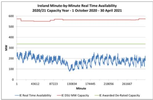
The use of the de-rating factors from previous determinations continues to ignore the increased adoption of short duration DSUs and their impact on the de-rating factors. Further to this, there also appears to be a mismatch between real-time availability and the de-rated capacity for DSUs (as shown above).
