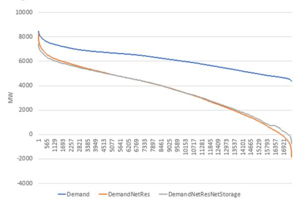
We then 'dispatch' unrestricted plant (and interconnection) against this duration curve, allowing 8 hours of insufficient capacity<sup>8</sup>. In the figure below we show the top 8000 half-hours (4000 hours).
