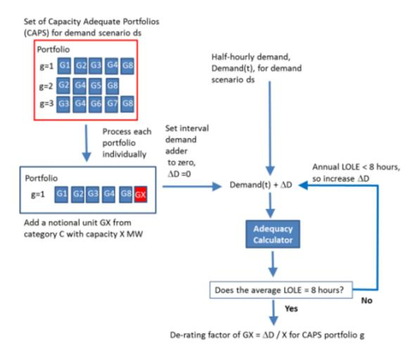
The marginal de-rating factor for a given technology and a given unit size is then defined as the ratio of the change in demand from a balanced position under a given adequate portfolio to get to the same LoLE level (<8 hours) and the capacity of the unit.
