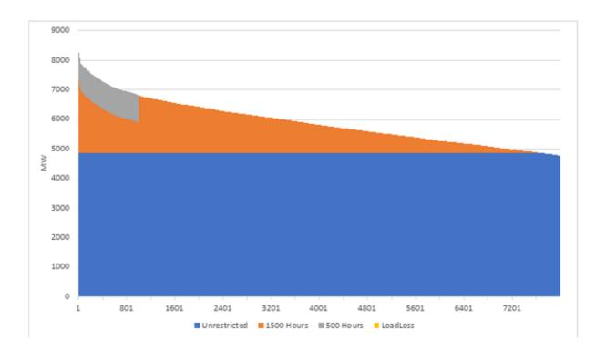
An unrestricted unit can reduce the hours the 1500h restricted unit needs to run by operating over all half-hours over which a limited hours plant would be otherwise running. This is 3845 hours. An incremental 1500h restricted unit could 'run' for 1500 hours and a 500h restricted unit could run for 500 hours. This suggests a marginal de-rating (in addition to normal outage/size de-rating) of:
